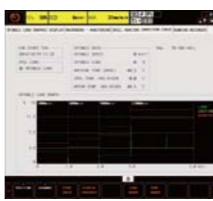
▲ Condition check Temperature as well as the motor load can be displayed.
