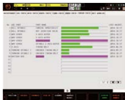
▲ Running recorder Operation status of milling spindle (rpm / motor load) can be recorded for up to one year.
