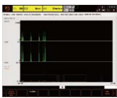
▲ Running recorder Operation status of milling spindle (rpm / motor load) can be recorded for up to one year.
