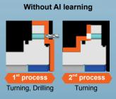
Interrupted cutting will be required in 2<sup>nd</sup> process which will affect finished surface.
