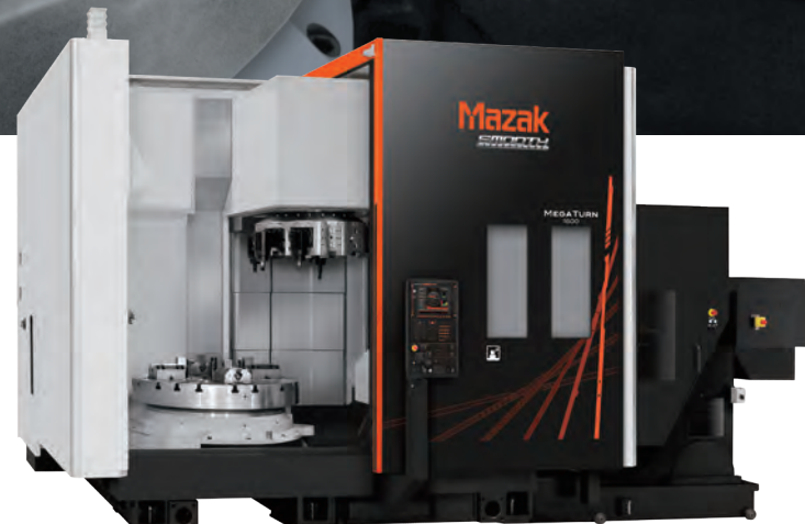
MEGA TURN 1600 (MAZATROL SmoothC) Shown with optional status light, ATC and chip conveyor
