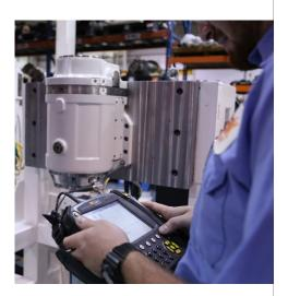
Regular spindle maintenance can help machine tool owners avoid or minimize the cost of a spindle repair. vibration. Increased vibration indicates worn spindle bearings, which, if ignored, can scorch spindle shafts and even cause spindles to seize during operation. Both of these scenarios are costly major repairs that could have been avoided by simply replacing worn bearings at the first sign of excessive spindle vibration.
