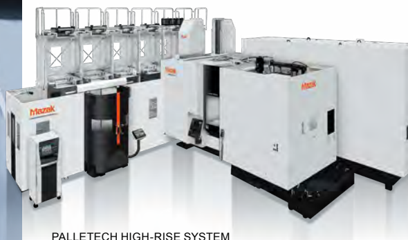
PALLETECH HIGH-RISE SYSTEM (3-level stocker with 18 pallets and one loading station)
