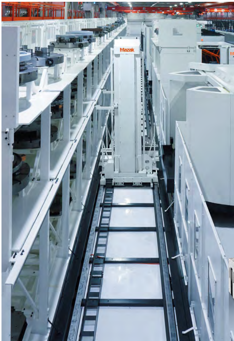
PALLETECH HIGH-RISE SYSTEM (3-level stocker with 18 pallets and one loading station)
