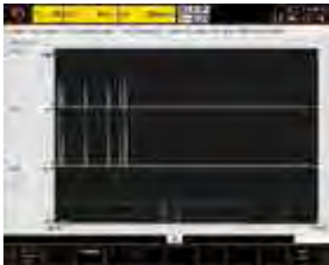
▲ Running recorder Operation status of milling spindle (rpm, % motor load and temperature) can be recorded for up to one year
