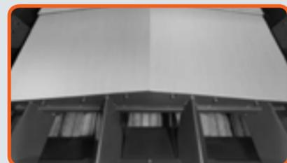
Enlarged chip ducts for smooth chip disposal
