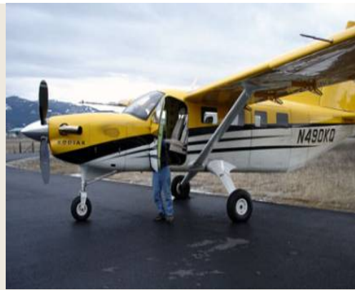
The Kodiak prototype following a test flight. It is a 10-place single-engine turboprop utility plane, also designed to be float-capable
