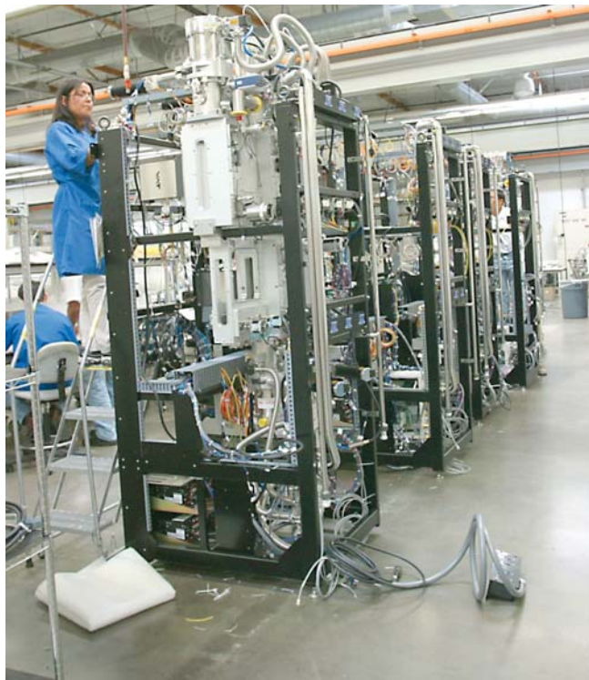
Four modules of the Intevac 200 Lean hard disk sputtering machine in process of being assembled.
