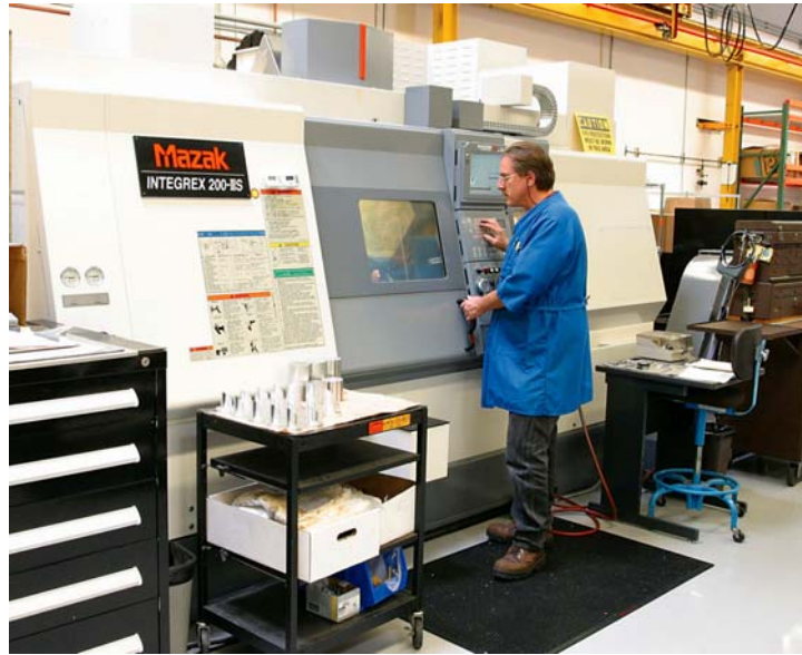
Shop leadman/programmer Diamond Hart sets up Intevac's Mazak 200-IIS multitasking machining center to run a prototype part.
