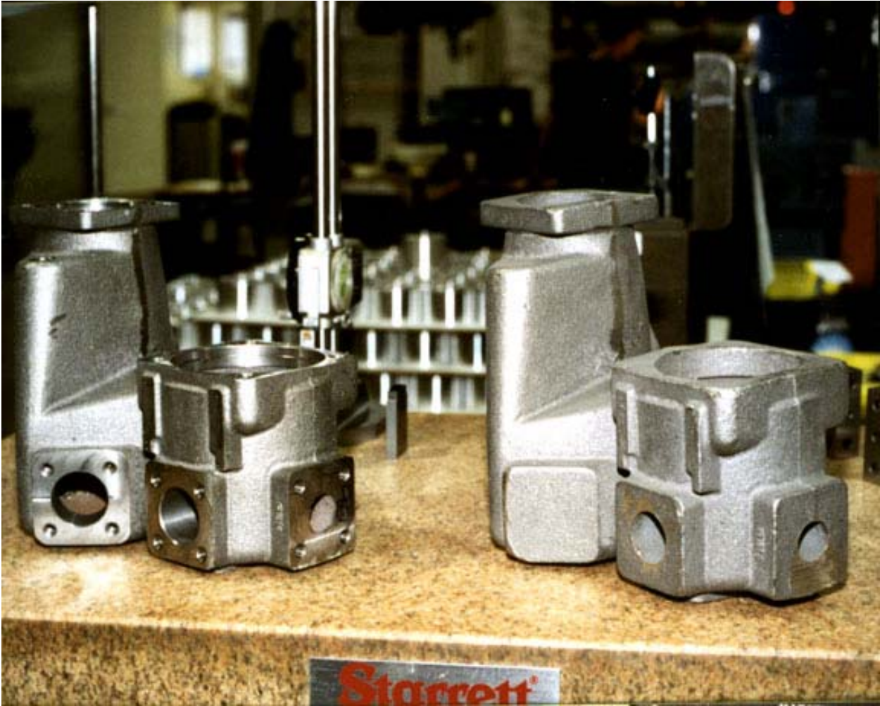
PHOTO CAPTION 2: Using the multi-axis capabilities of the Variaxis 200, Liqua-Tech cut machining times in half on this iron casting for its LPM-102 liquid propane flow meter.
