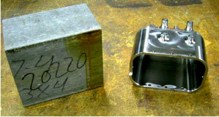
An aerospace component is machined from a solid on Mack's Mazak equipment.
