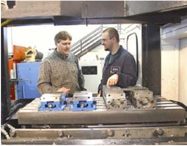
Caption: RPM partner Shawn Bindrup (left) and CNC operator Justin Bassett discuss the most efficient set up on the Nexus 510C dual-pallet system. Note the wide open, easy access to the pallets from both sides of the machine. RPM has made major productivity gains since installing the Nexus.
