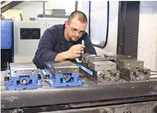
Caption: CNC operator Justin Bassett checks set up on the Reed Precision Machining's Nexus 510C dual-pallet system. Note the wide open, easy access to the pallets from both sides of the machine. RPM has made major productivity gains since installing the Nexus.
