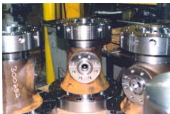
Valve bodies such as these require multiple operations on multiple faces, making them great candidates for multitasking.
