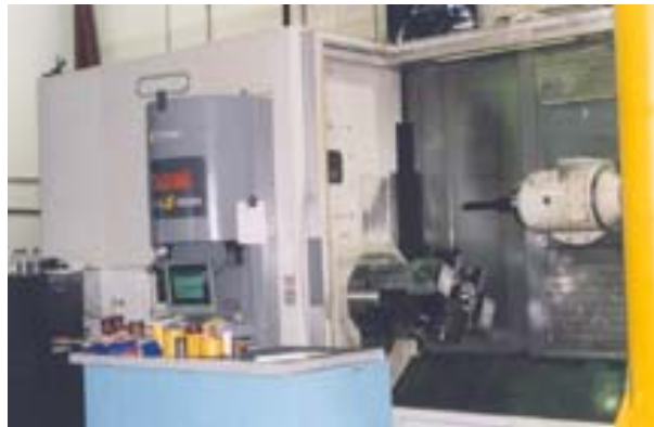
Domino's Integrex e650H with an indexing chuck is the first of its kind in North America.
