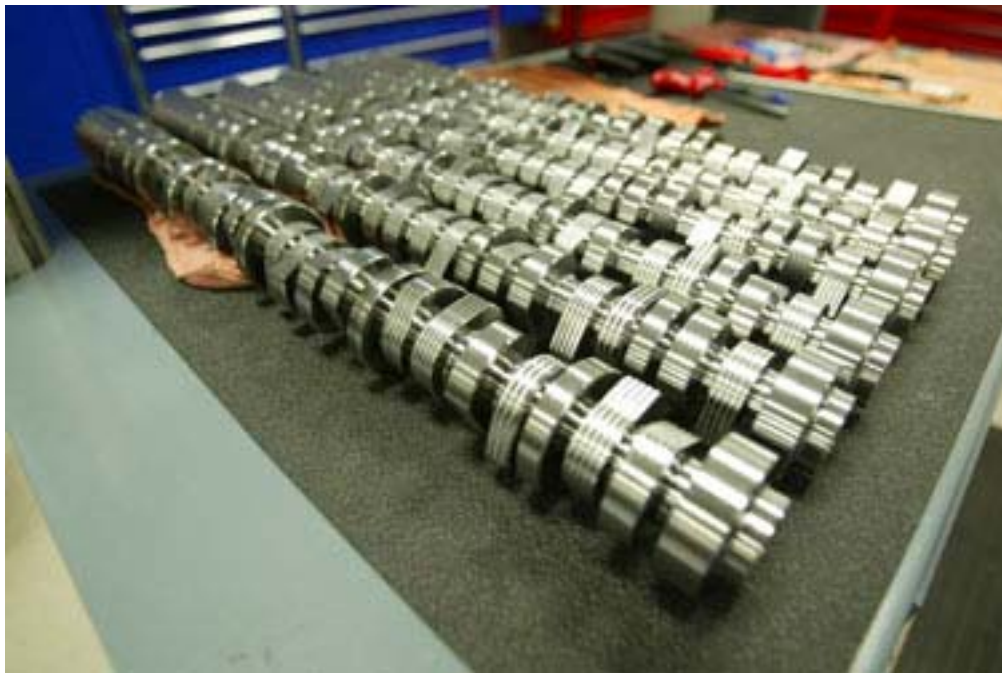
Photo caption: Making and testing custom camshafts means Penske Racing South has more options to fine-tune engines for specific tracks and racing conditions.
