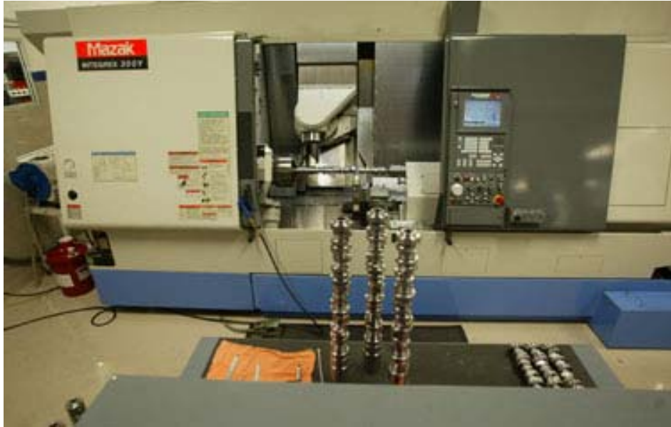
Photo caption: Making and testing custom camshafts means Penske Racing South has more options to fine-tune engines for specific tracks and racing conditions.
